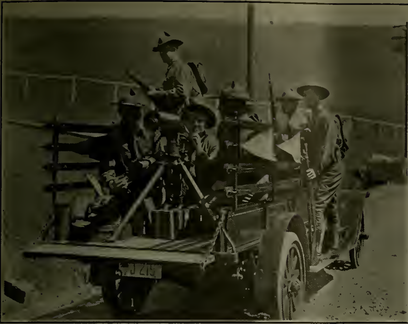
Maxim Machine Gun, mounted on Kissel Truck, 1 ton worm drive, at Fort Baker Photo by Arthur Spaulding Co., San Francisco.
